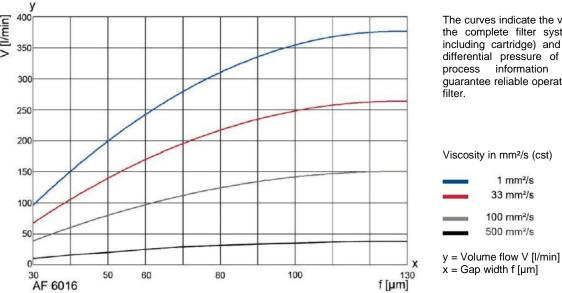
The curves indicate the volume flow through the complete filter system (filter housing including cartridge) and are referred to a differential pressure of 0.3 bar. Specific information is essential guarantee reliable operation of an automatic
