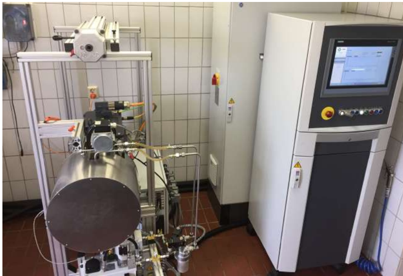
BECHEM FE 8 test rig
