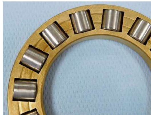
Cage and rolling elements after the test
